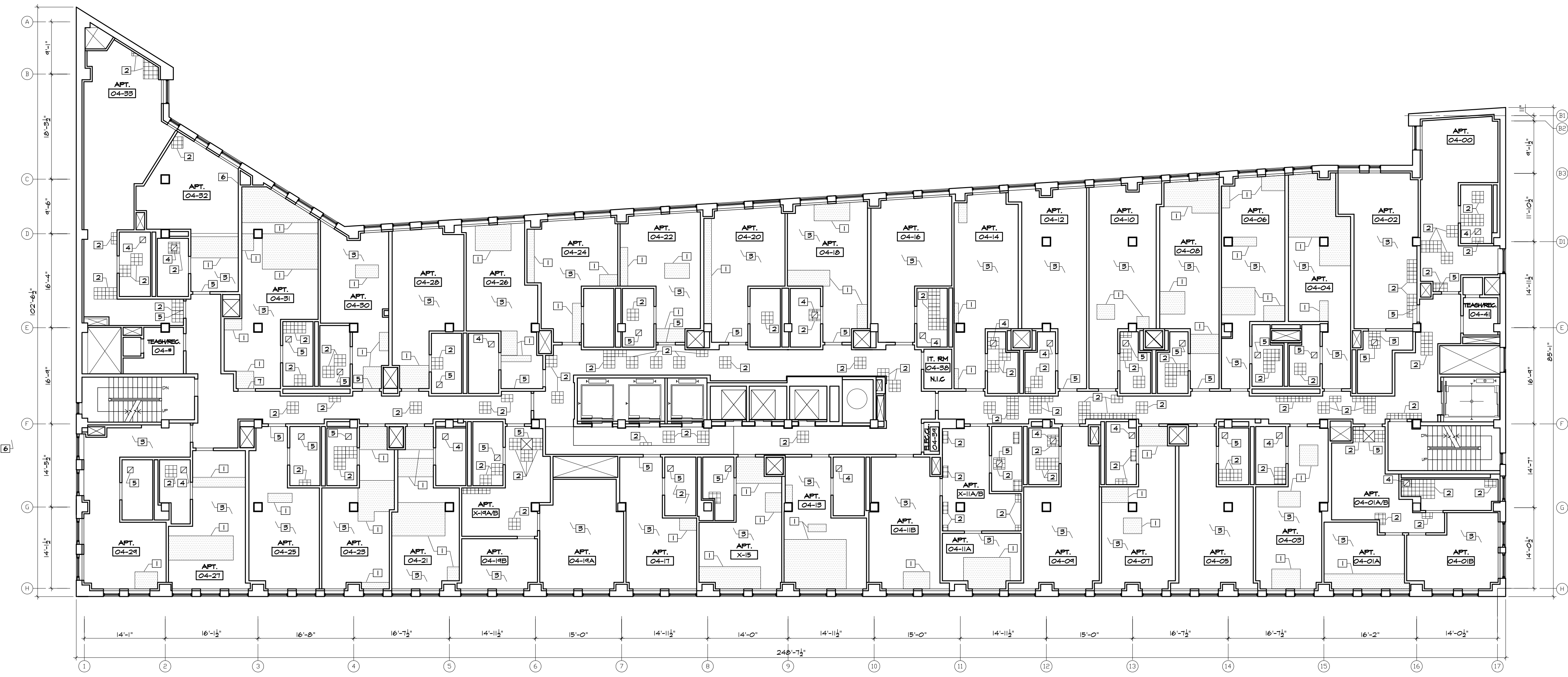
1 4TH FLOOR RCP CEILING REPAIRS A-403 SCALE: 3/32" = 1'-0"
