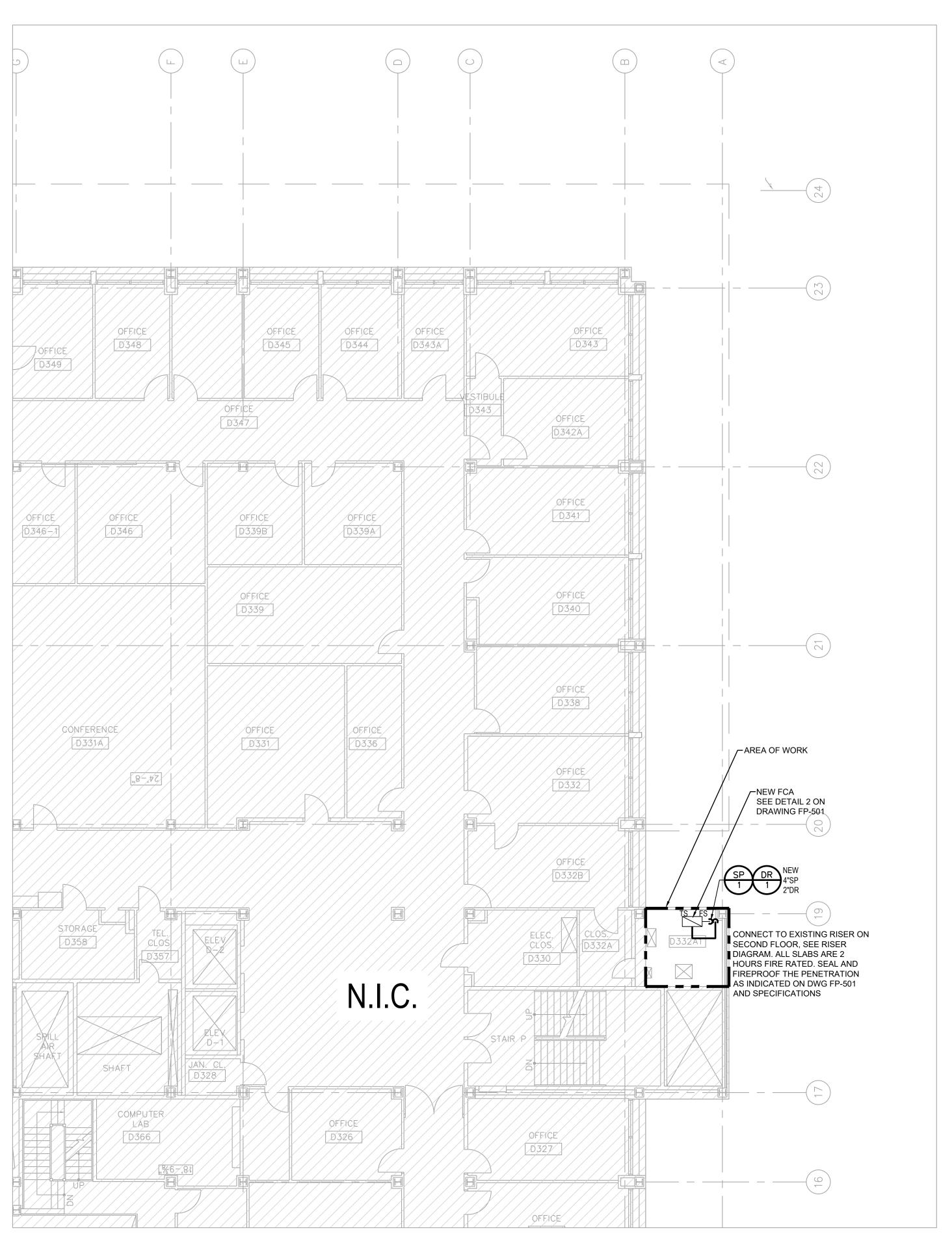
1 TYPICAL FLOOR (3RD, 4TH, AND 5TH) PARTIAL FIRE PROTECTION PLAN
